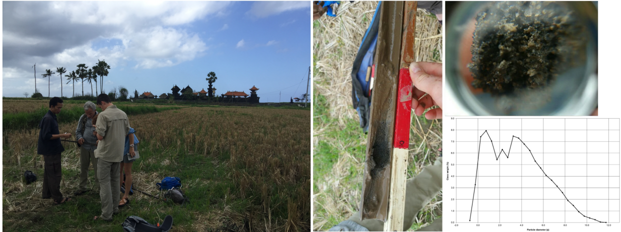
Figure 9. Left: photo of the coastal plain in Rangan Beach. Middle: sand layers identified from augur. Right: Grain size distribution of the sand.
