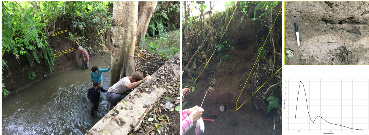
Figure 7. Left: photo of the river bank in Purnama Beach showing sand layers. Middle: 2 sand layers identified on the field. Right: Grain size distribution of each sand layers.
